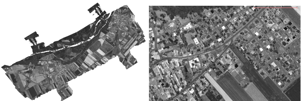
Figure 2: Upper image: Calibrated reflectance image (1550 nm) of the complete study area Carnuntum (Briese, Pfennigbauer, Ullrich, Doneus, 2013); Lower Image: Detail of the reflectance image; the length of the red line in the upper right part of the image represents 200 m. In both visualizations the reflectance images (255 gray values) are linear scaled from 0 (black) to 0.5 (white)
