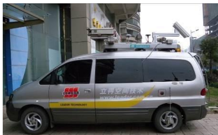
Figure 10: Detection of pavement cracks MMS
