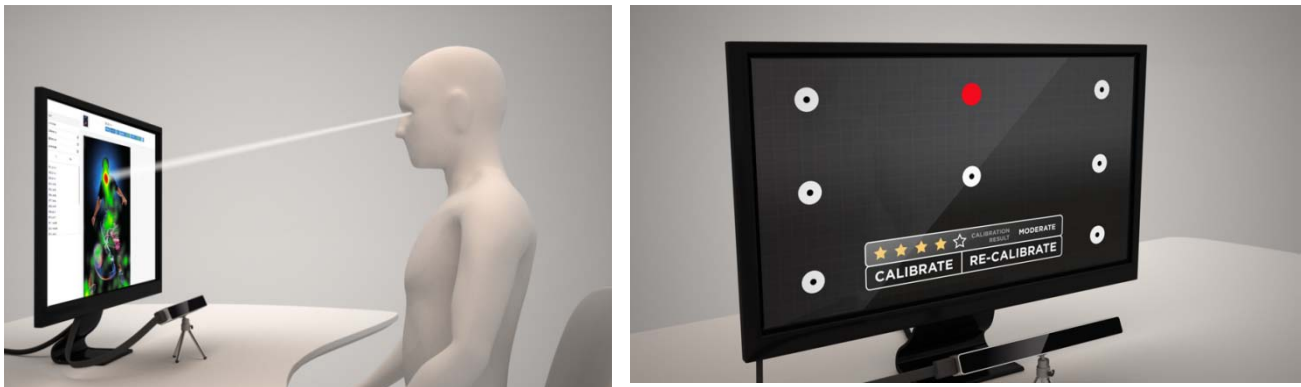
Figure 1. a) The Eye Tribe System b) Calibration process screen (TheEyeTribe)
