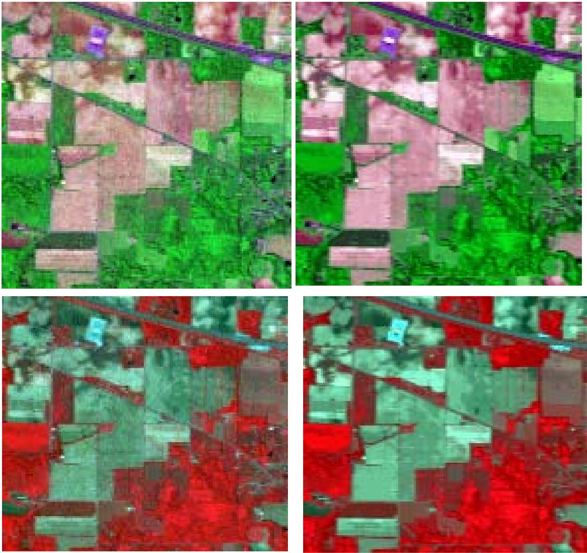
Figure 2: Original (left) and Noise-reduced (right) color composites of a hyper-spectral AVIRIS images. Above: channels (177, 77, 17) mapped to RGB, below: channels (42, 22, 10)
