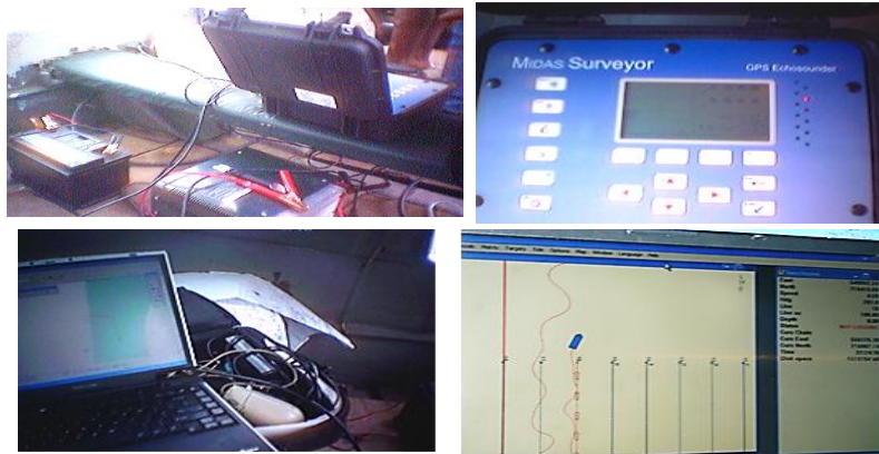
Fig. 2. Survey Boat, MIDAS Surveyor Echo Sounder, Toshiba Laptop and Hypack Navigation System software window. Source [5]
